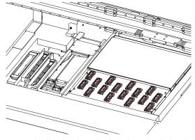
The NCU (Nozzle Check Unit) automatically checks whether the nozzle is clogged. Setting various functions enables automatic print head cleaning or printing using other nozzles. "Nozzle Check Before Print"(P. 119)
