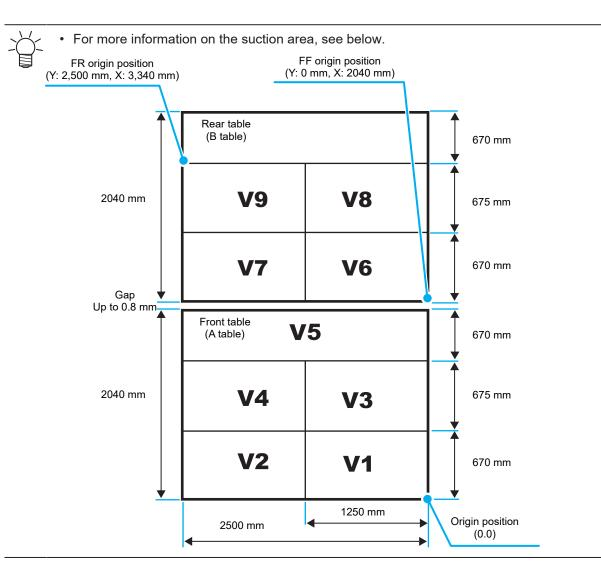
From QUICK MENU on the touch panel, tap [Vacuum] or step on the foot switch to apply suction to the media.
