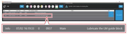
• The frequency with which the alarm is displayed is generally determined by the distance traveled by the machine, but this depends on the machine usage. (Distance of 450 km: Equivalent to approx. 2 years)
