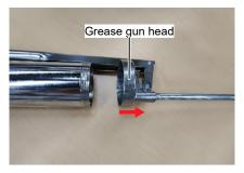
(2) Insert the grease cartridge.
