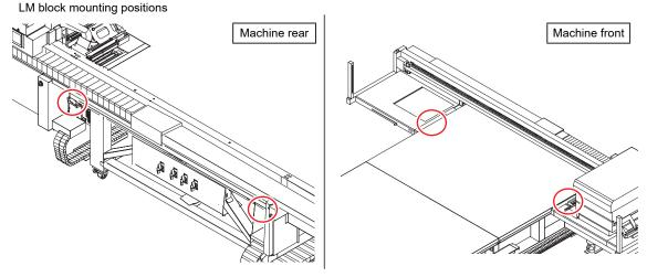
• Push the grease gun on to the grease nipples to lubricate. (Greasing guide: 2 pushes)
