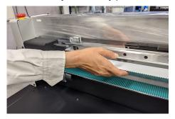
Keep your face, hands, and all other body parts at a safe distance from the cable carrier section, and do not place any objects on top.
