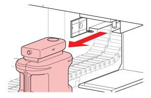
Attach the cap to the removed waste ink tank, and use tape to prevent leakage of waste ink.
