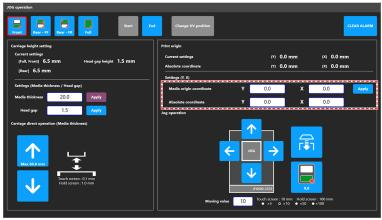
• Absolute coordinates: The coordinates from the origin at the lower right corner of the table (<Y,X>=<0,0>) are displayed as absolute coordinates. For example, the media origin coordinates (<Y,X>=<0,0>) in [FF - Rear] mode correspond to the position (<Y,X>=<0,2040>) when expressed in absolute coordinates. Similar to the media origin coordinates button, selecting the button executes the specified value movement.
