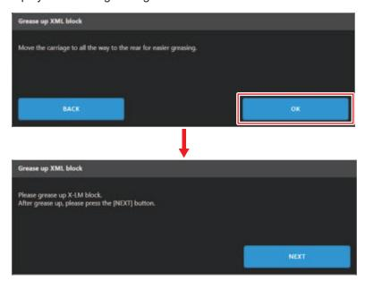
3 Check to confirm that this is the greasing window, then lubricate the four LM blocks.
