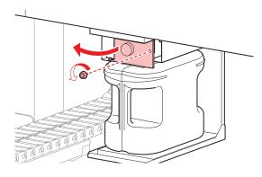
▲ Grasp the handle of the waste ink tank and slide out.
