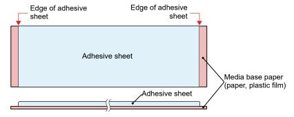
(1) Make sure there is no pinch roller within 10 mm from the edge of the adhesive sheet and that the pinch roller is not in contact on the grit roller.
