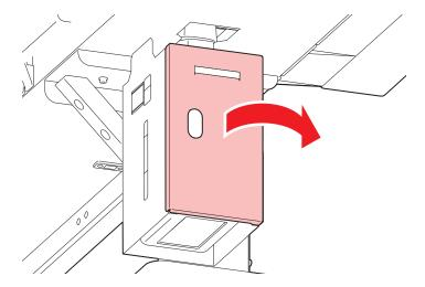
▲ Hold the handle on the waste ink tank and slide out.
