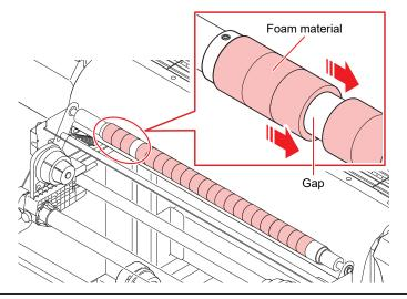
If the foam material on the bonding roller is not in the correct position, move it into position as follows.
