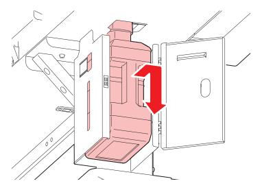
5 Attach the cap to the removed waste ink tank, and use tape to prevent leakage of waste ink.
