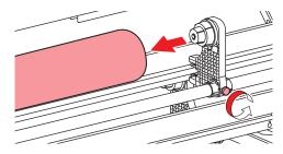
6 Tighten the retaining screw on the rear right roll holder.
