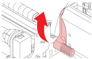
(2) Take the side of the cut release paper that faces the rear of the machine and route it between the pinch and grit rollers. (This is to move it out of the way, behind the machine.)
