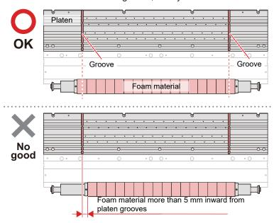
(2) Also move the foam material if there are any gaps between individual pieces of material. If the foam materials hit each other strongly, bubbles are likely to occur during crimping. Once the gap between the foams is gone, do not press any harder.
