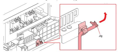
• Connect the jig by pushing the tip into the port and rotating 30° clockwise.
