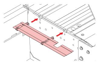
7 Secure the media holder stopper with the screw.
