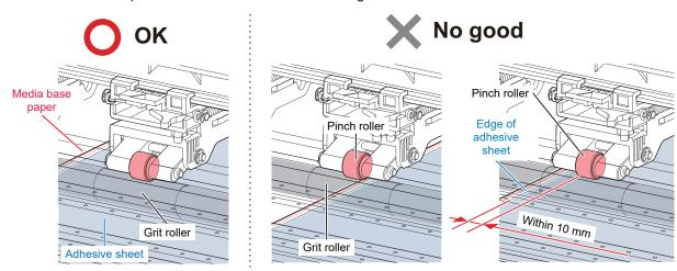
(2) Pinch rollers not in proper position, contact may cause adhesive sheets to get caught in pinch rollers. Move the clamp change lever to raise the pinch rollers.
