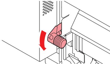
**10 Move to the front of the machine and open the front cover.****11 Raise the clamp lever and pull out the media.**
