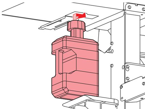
**8** Close the waste ink tank stopper.
