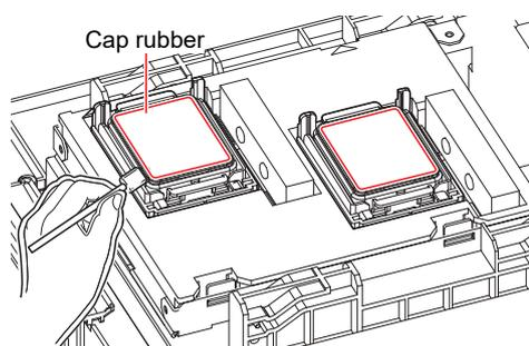
**5** Check to confirm that the cap slider is not tilted once cleaning is complete.
