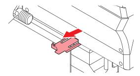
Hold the handle on the waste ink tank and slide out.
