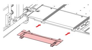
7 Secure the media holder stopper with the screw.
