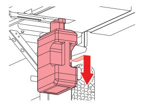
Attach the cap to the removed waste ink tank, and use tape to prevent leakage of waste ink.
