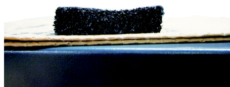
Ink absorption material that requires replacement (deformed)
