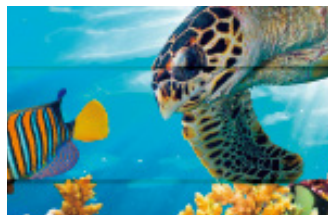
Overlap/Black streaks (Insufficient feeding amount)
