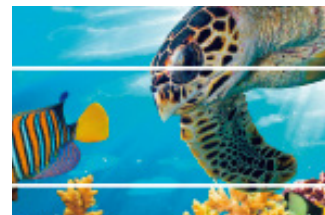
Gap/White streaks (Excessive feeding amount)
