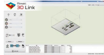
For 3D print job layout and transmission to the printer
