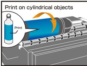
Mount Kebab MkII / MkII L option to the printer and set the cylindrical object on the rollers of this option. Using the special software will automatically start printing on the entire 360° surface of your desired object. The option can be easily mounted onto the printer using the special plug and the fixing screws.
