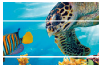
Gap/White streaks (Excessive feeding amount)
