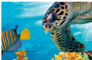
Overlap/Black streaks (Insufficient feeding amount)
