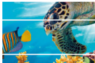
Gap/White streaks (Excessive feeding amount)
