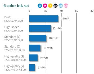
\*When printing with Sb420 dye sublimation ink. DD400,TP400, Rc400 inks cannot print in draft mode
